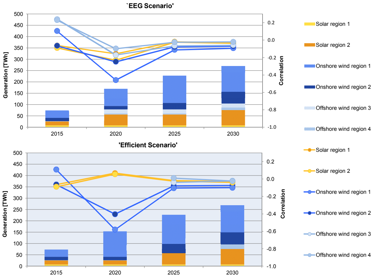
Figure 5: Annual generation [TWh] and annual correlation between the wind/solar power generation profile and the wholesale price profile
