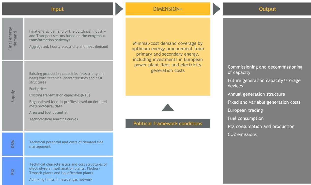
FIGURE 57: SCHEMATIC REPRESENTATION OF MODEL OF THE ENERGY INDUSTRY
