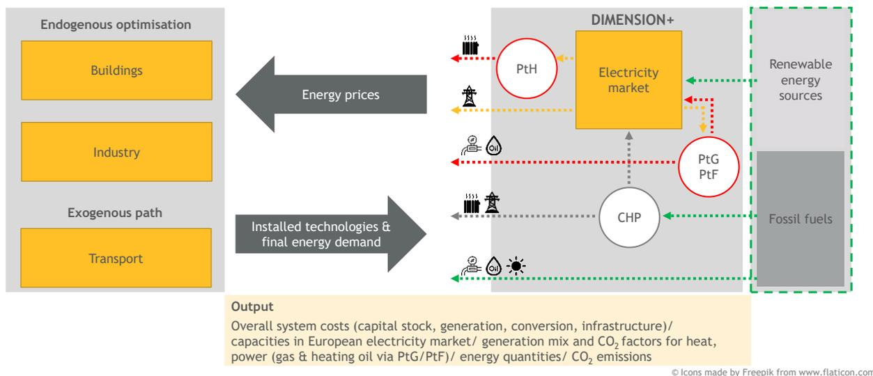
FIGURE 56: SCHEMATIC DIAGRAM OF THE DIMENSION+ ENERGY SYSTEM MODEL
