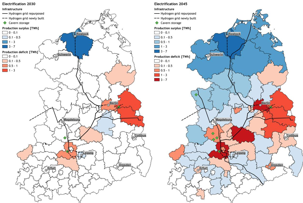
Figure 6: Potential hydrogen grid in the *Electrification* scenario for 2030 (left) and 2045 (right)
