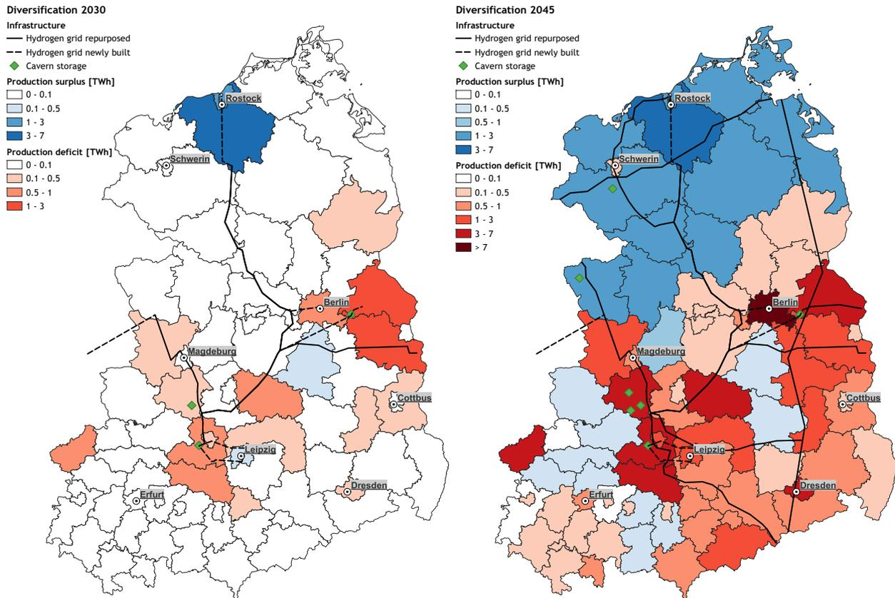
Figure 7: Potential hydrogen grid in the *Diversification* scenario for 2030 (left) and 2045 (right)
