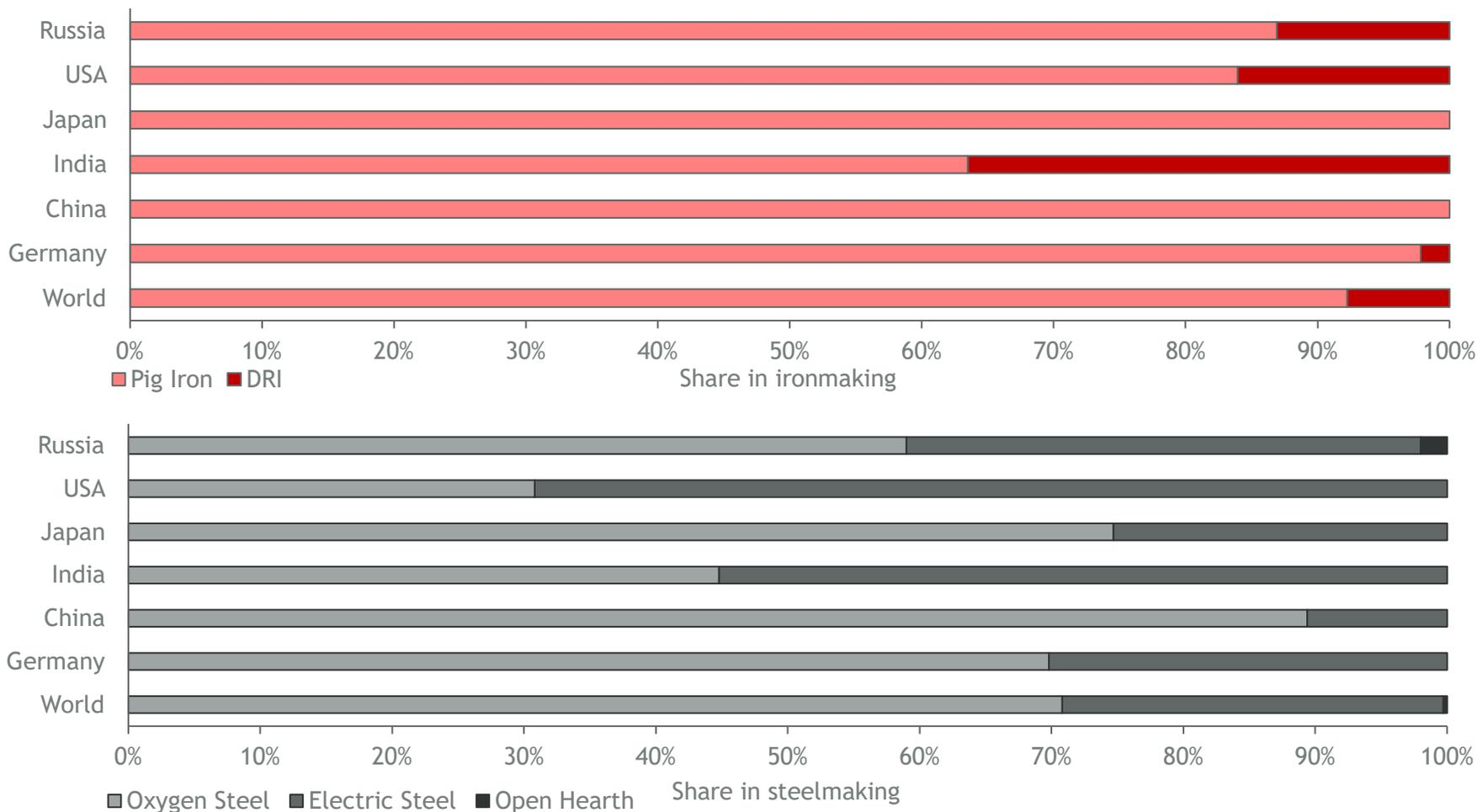
Figure 3: Technology shares for ironmaking (top) and steelmaking (bottom) in 2021 globally and for selected countries.
