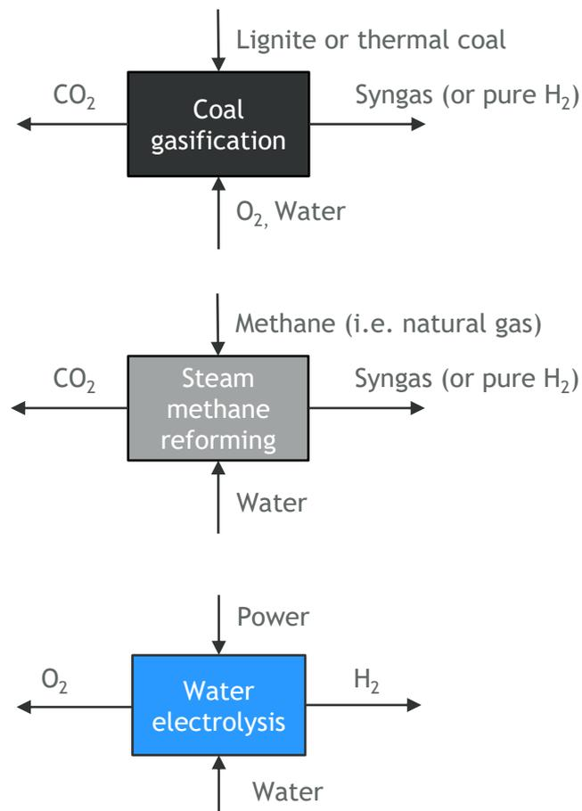
Figure 7: Flowsheet of essential mass and energy flows of a water electrolysis, coal gasification and steam methane reforming process.
