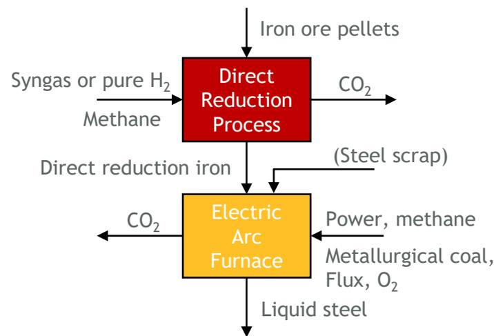
Figure 6: Flowsheet of essential mass and energy flows in an integrated direct reduction process & electric arc furnace steel plant.
