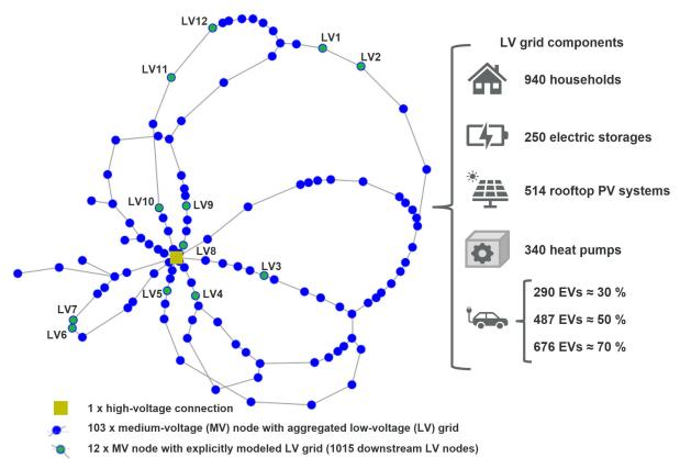
Figure 4: Configuration of the distribution grid
