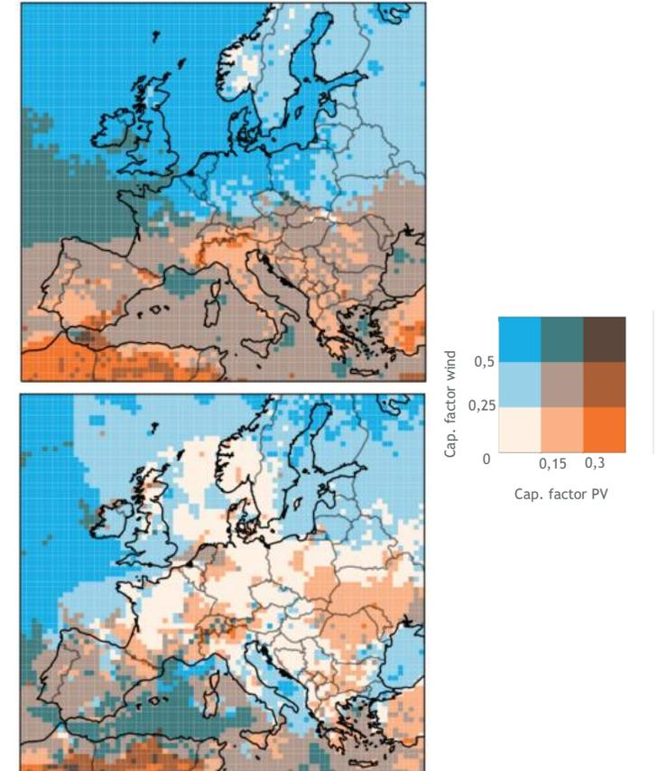
Figure 17: Capacity factors for wind and PV generation - 1995-2014 long term mean of winter (DJF) (top) and January 1997 (bottom)
