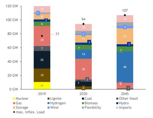
Figure 16: Development of inflexible peak demand and provision of firm power plant capacity by energy carrier
